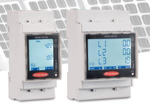
The Fronius Smart Meter TS is a bidirectional meter, which optimises self-consumption, records the load curve and controls the various energy flows. Thanks to highly accurate measurements and rapid communication via the Modbus RTU interface, dynamic feed-in control when feed-in limits are imposed is faster and more accurate than with the S0 meter.
